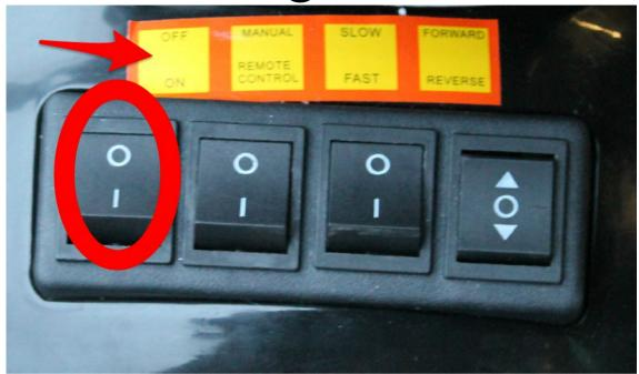
To turn the Quad on, please make sure that the highlighted switch is in "I" position.
